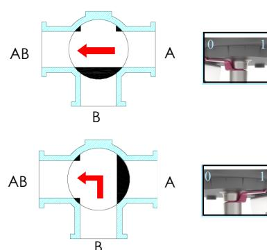
When actuator pointer tends to “0”, the flow increases from A to AB and decreases to A.
