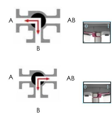
When actuator pointer tends to “0”, the flow increases at A and B and decreases at AB.
