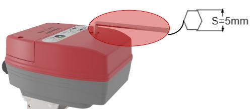
3. Turn the Allen wrench counterclockwise, the valve is closed from AB to A and opened from AB to B.
