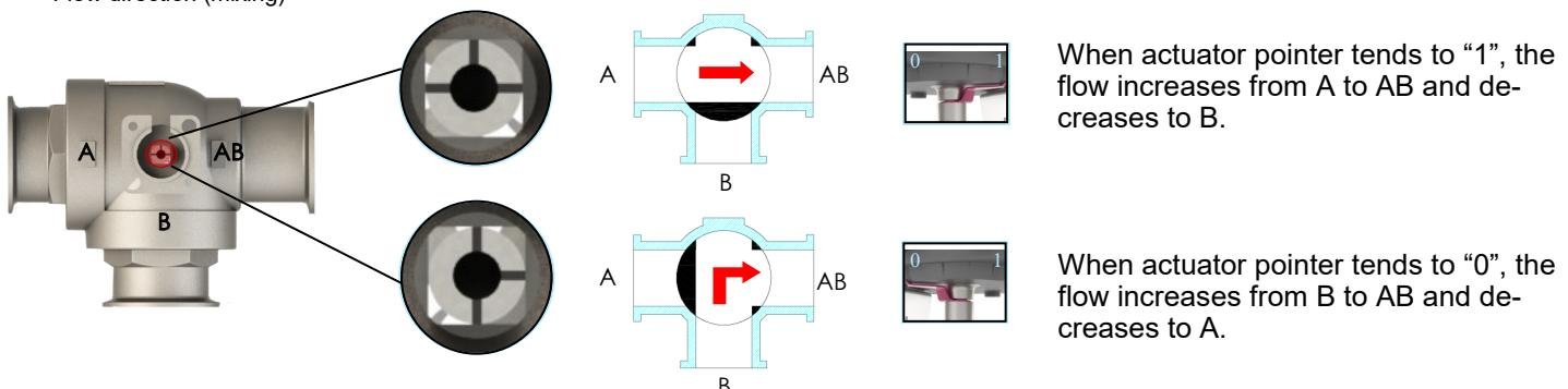
When actuator pointer tends to "1", the flow increases from A to AB and decreases to B.
