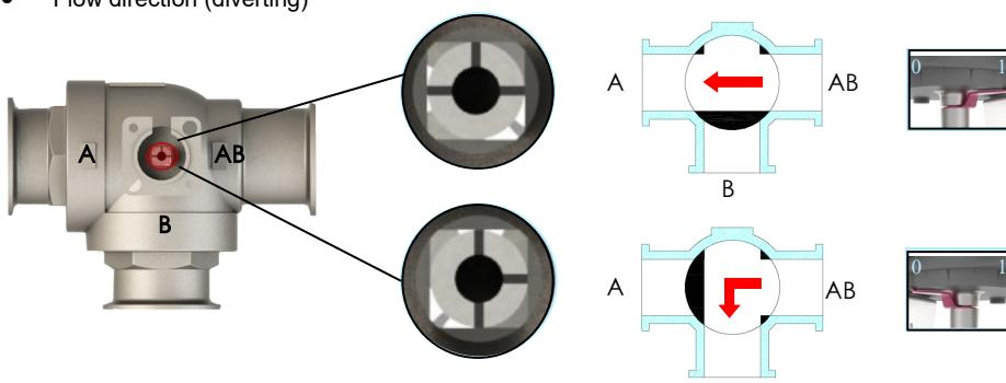
When actuator pointer tends to "1", the flow increases from AB to A and decreases to B.
