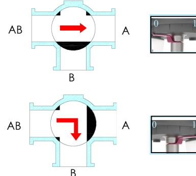
When actuator pointer tends to “0”, the flow increases from AB to A and decreases to B.
